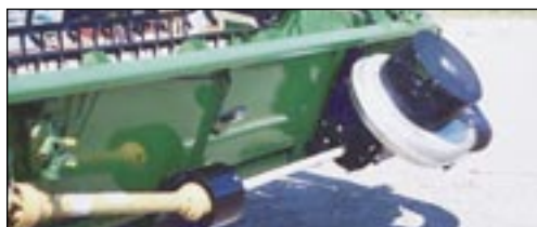
The fan is driven by either a gear box or belt drive system featuring a heavy duty PTO drive shaft with slip clutch.
