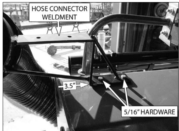
Figure 32, Hose connector weldment
